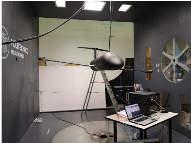
GVT session inside the WT chamber, the final hybrid FEM model, and the anti-flutter safety device
