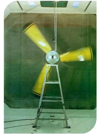
3 bladed HAWT model (D=2m) in section 1
